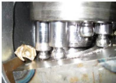
Axial pump damage due to cavitation
