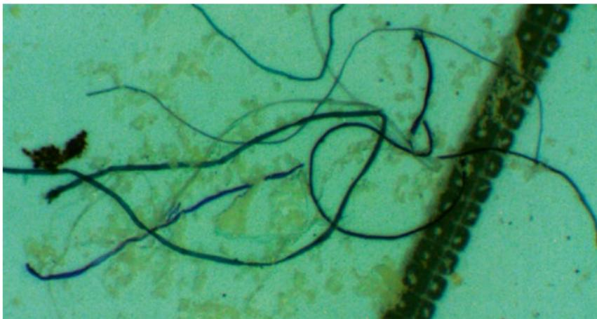
100x magnification of a sample of unfiltered HLP 46 fresh oil as supplied in a canister
