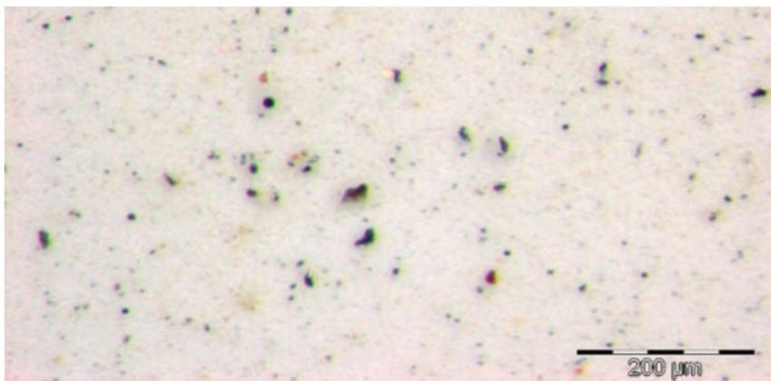
ISO code 21/19/16 – the minimum requirement for fresh oil supplied in accordance with DIN 51524
