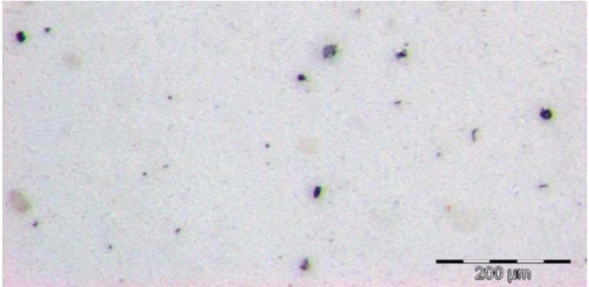
ISO code 19/17/14 – requirement for electromagnetic control valves
