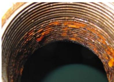
Corrosion of threaded connections on a hydraulic tank due to high atmospheric moisture content
